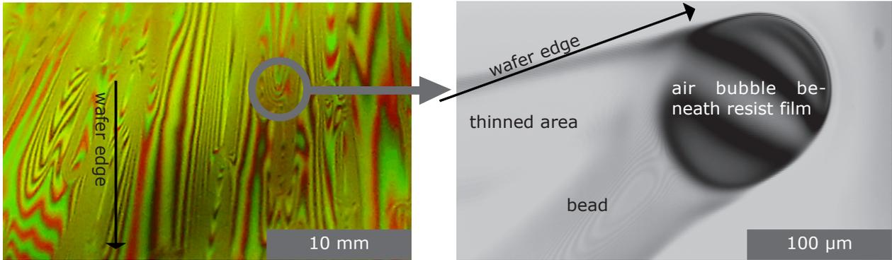
Inhomogeneities in the coated resist film (left) often misinterpreted as particles, mostly originate from air or N<sub>2</sub> bubbles (right).
