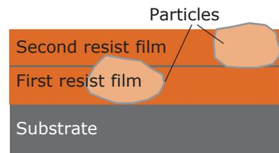
Double coating can only be realized with high-viscosity resists, since a high solvent concentration will cause a dissolution of the existing resist film. The lower the resist viscosity is, the more important is i) a softbake between the two coating steps, and ii) spin-coating immediately after the second resist dispensation in combination with a high acceleration in order to suppress the dissolution of the first resist film.
