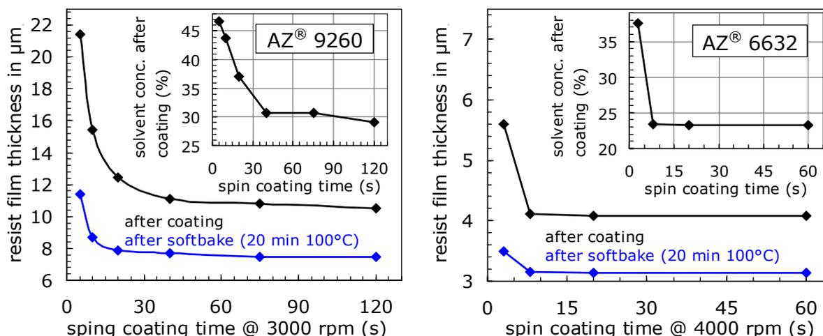
Resist film thickness and remaining solvent concentration after different long spin coating for a thin (left) and thick resist (right) before (black) and after (blue) softbaking.
