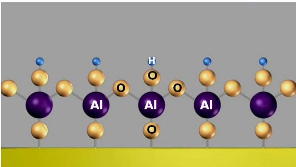
**Step 4: Removal of the unreacted precursor and reaction products via evacuation and/or inert gas flow.**
